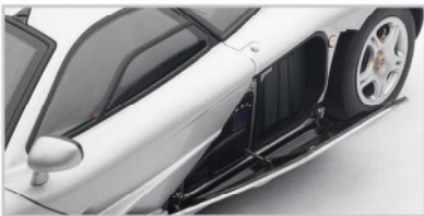
Gold and silver foil are applied on the underneath of the three working engine covers, as well as the area around the engine bay.
