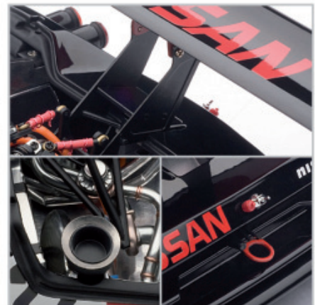
Precised machine cut metal are used for the supporter of rear spoiler, suspension, full filler neck and tow hook.
