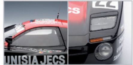
More than 80 pieces of tiny rivets are applied on window frame, headlamp covers and body panels manually piece by piece which indeed a costly process.
