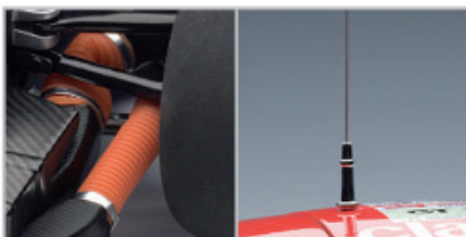
Rubber cooling pipes for braking system are used. Metal aerial on the roof.
